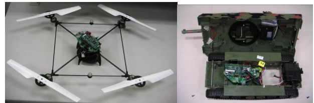
Figure 16 – Quadrotor (Left) and Tank (Tight) Test Vehicles Use Boeing Common Hardware.
