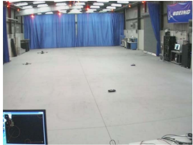
Figure 18 – Heterogeneous Area Coverage Test in VSTL. Mission Planner is Shown in Bottom Left.
